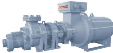
CO 2 Semi-hermetic screw compressor with adjustable volume ratio and permanent magnet variable frequency drive
